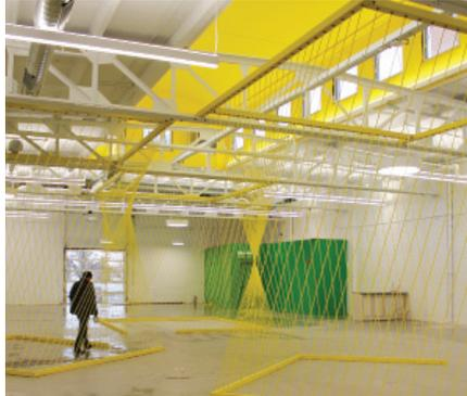
The bright yellow bungee cord enclosures are also designed to encourage movement, he added. Each bungee cord is angled along a track producing what is termed a ruled surface, resulting in a sense of undulation, even though the strands are all perfectly straight.
